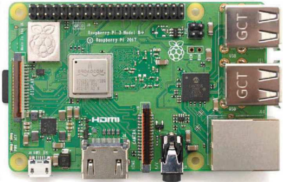
A new, smarter PMIC chip means a simplification to the board layout and a reduction in the overall component count
